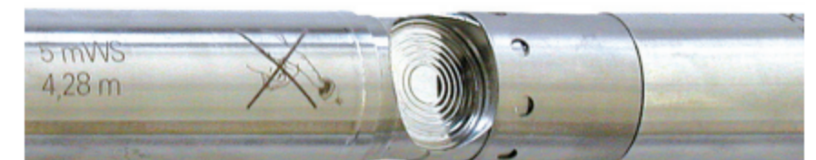
Integrated air pressure sensor with diaphragm protection
